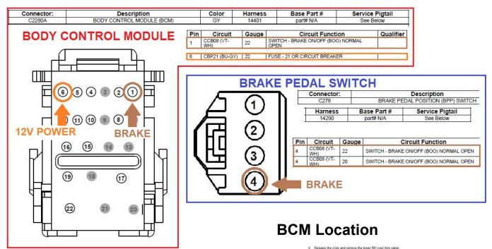
The BCM is located in the passenger foot well behind the interior trim panel.
